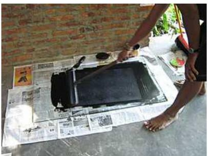
Once all surface is well inked, it is time to roll the textile on the wooden plank: it has to be done **carefully** so that there are no wrinkles left. While proceeding unrolling the textile, the surface of the textile must be immediately covered with paper.
