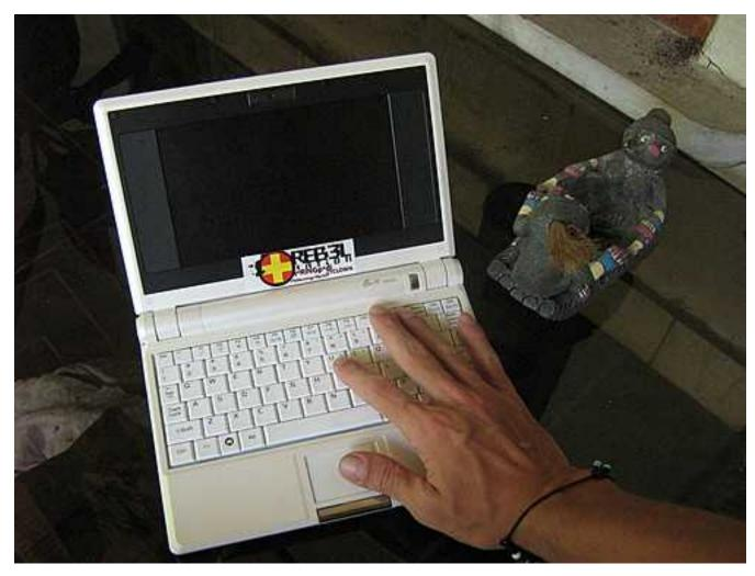
The best feature consists in being completely **solid state**: no mechanical parts moving, which means more robust and less energy consuming. It is equipped with a Pentium M with 512 of RAM and 4GB NAND (internal storage), has wifi modem and ether-net, an SD card slot, usb2.0, sound-card and even a web-cam.
